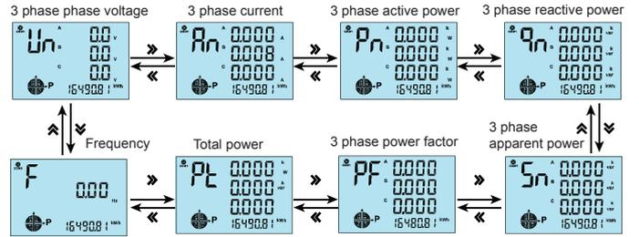
(note: in 3 phase 3 wire status only display 3 phase line voltage, current, total active power, reactive power, total power factor, frequency )
