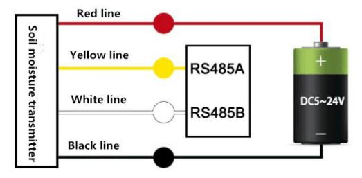
Note: The shielded cable (green line) is connected to the power supply for the acquisition mode, and the power supply is in the setup mode.
