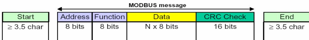
A typical Modbus RTU mode message frame is shown as above. In the Modbus RTU mode, the messages between frames are separated by at least 3.5 characters time's silent interval. If the silent interval between two characters is more than 3.5 characters time, the former character was transferred successfully, and the current character's transmission starts.
