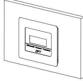
(1) Cut a 95(W)×80(H)mm rectangular hole on the wall.
