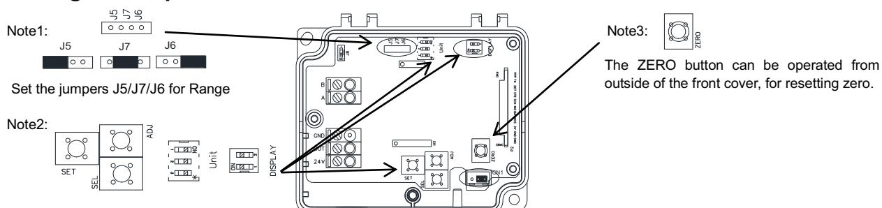
1. Unit setting: Set the unit switch as below.
